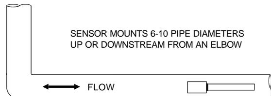
**PIPE MATERIAL** - Sound conductivity varies according to the density of the pipe wall material. Porous materials such as concrete or wood cause sound attenuation and Doppler performance may be erratic. Steel, PVC, cast iron, copper, aluminum, fiberglass and other plastic and metal pipes are generally ideal, with minimal sound attenuation.
