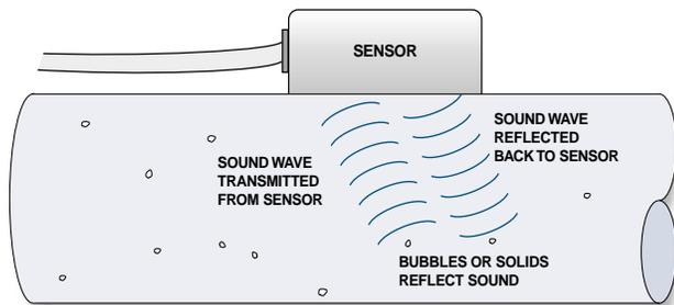
The advanced DFM sensor contains two piezoelectric crystals in a stainless steel housing. One crystal transmits ultrasonic pulses at a precise frequency which are reflected back to the receive crystal from gases or solids in the liquid. Because the fluid is in motion the returned echo arrives back at the sensor at an altered frequency (called the Doppler effect). The instrument's electronics monitor and convert this frequency change into velocity flow readings.
