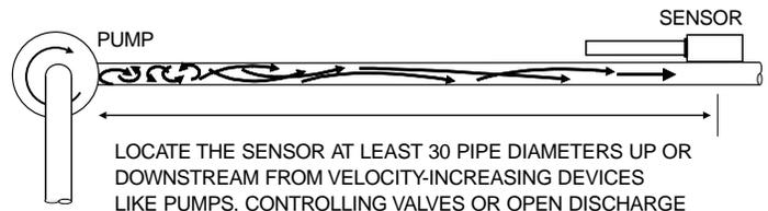
Elbows, flanged connections and tees introduce desirable conditions of an evenly distributed flow profile with some air or gases entrained in the flow. Sensor mounting 6 to 10 pipe diameters up or downstream from these disturbances is generally optimum.
