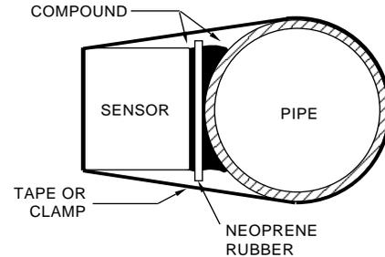
**SENSOR POSITIONING** - The sensor must be mounted away from velocity increasing devices such as pumps, controlling valves, orifice plates, venturis, or pipe inlets and discharges. These devices cause release of gas bubbles in the fluid and readings nearby will indicate higher velocity. Normally flow will be evenly distributed 30 to 40 pipe diameters away from the velocity increasing device. Determine an appropriate up or downstream sensor mounting location by onsite experimentation.
